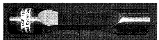
Notch : Width & Depth = 0.25mm
