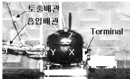
Fig. 7 Experimental setting of linear compressor
