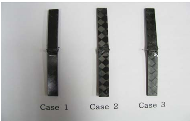
Fig. 6 Failure configuration after compressive specimen tests
