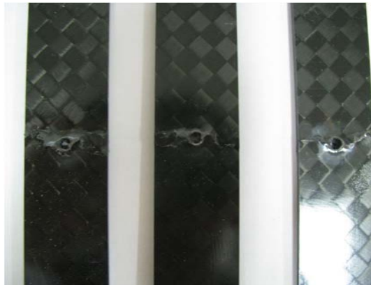
Fig. 9 Failure configuration after compressive specimen tests
