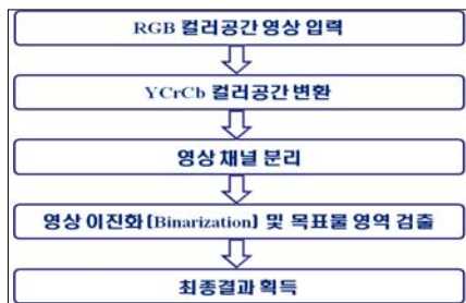
Fig. 12 Procedure of Image Processing
