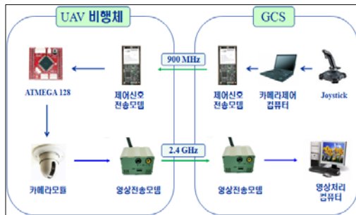
Fig. 7 Concept of EO Sensor Module System
