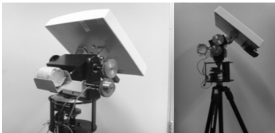
Fig. 8 Antenna Tracking System Frame
