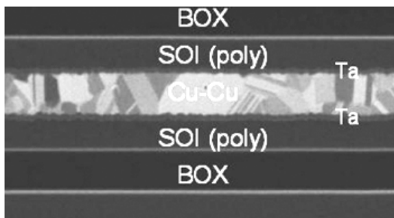
Fig. 4 FIB image of Cu to Cu bonding 4)
