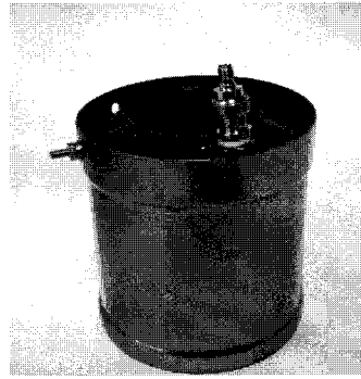
Fig. 3 PLC Coupler without matching circuit
