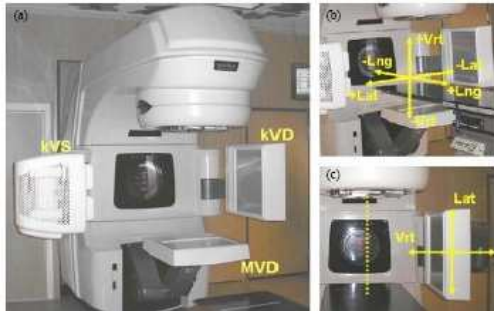
Fig. 1. (a) Varian clinical linear accelerator with an On-Board Imager(OBI) consisting of two robotic arms; one holding a flat panel imager(kVD). The mega voltage detector(MVD) is also extracted. (b) The coordinate system for couch/patient position: Lat = + Right/-Left, Vrt==Ant/-Post and Lng =+ Inf/-Sup. (C) Lateral and vertical motion of the kVD are relative the MV beam axis.
