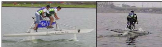
Fig. 2 Unstable human powered hydrofoil boat
