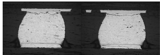
Fig. 10 Cross-sectional micrograph of a solder ball with crack
