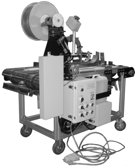
Fig. 7 Picture of the prototype of the automatic bundling machine
