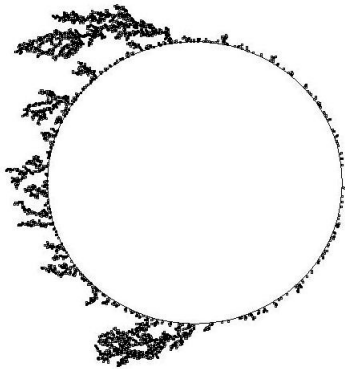
Fig. 8 When d_p=0.05\mu\text{m} , morphology of particle deposit layer
