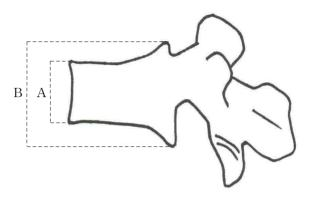
$\begin{array}{l} compression \ ratio = \\ (1 - Anterior \, wall \, height \, (A) / Posterior \, wall \, height \, (B)) \times 100 \end{array}$
