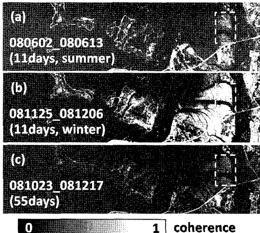
Fig. 5. Coherence map of summer pair (a) and winter pair (b). Winter pair shows much better coherence. (c) The areas of halophyte (boxed area) maintains coherence even with long time interval.
