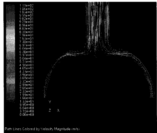
Fig. 10 Flow pattern of flat impingement plate at center section of inlet nozzle
