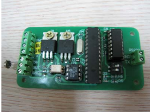
Fig. 6 Water temperature sensor and data acquisition system
