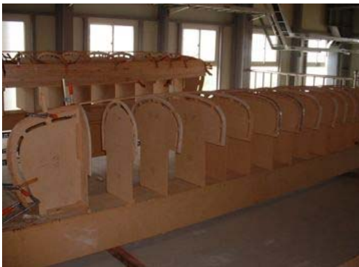
(a) Preparing section molds and die of a hull
