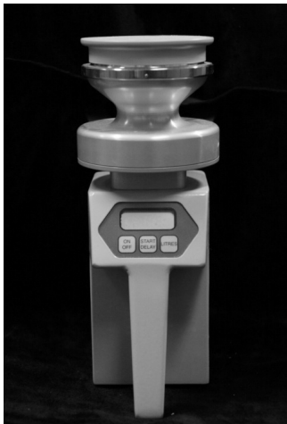
Figure 1. Air sampler (M Air T TM , Millipore Corp., Massachusetts, USA) for inhaling the aerosols produced by ultrasonic scaler before, during or after the treatment. The trypticase- soy agar plate is installed at the entrance of the air sampler.
