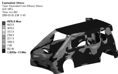
Fig. 20 Contour of Equivalent Stress at Car in Case of Double Impact (Elapsed time of 0.004sec)
