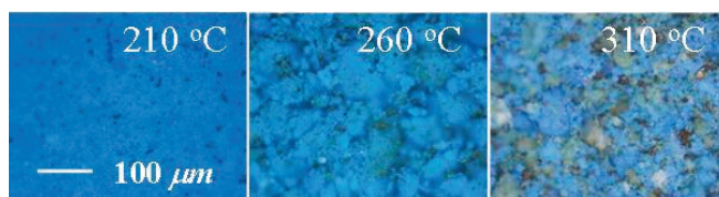
Figure 6. Optical images of the samples obtained by decomposing the 35-precursor at 260 and 310 °C.
