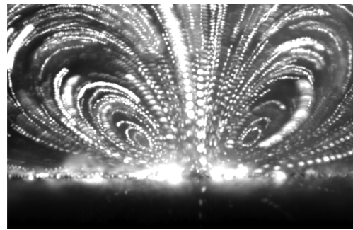
Fig. 3. AC Electro-osmotic flow generated by a pair of coplanar electrodes. (a) Schematic diagram of the set-up; (b) typical flow pattern near the electrodes.
