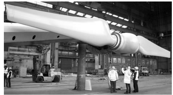
Fig. 3. Rotor and blade of SeaGen turbine with the capacity of 1.2 MW [38].
