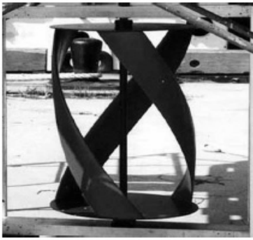
Fig. 4. Gorlov Helical Turbine equipped in Uldolmok (The rights to the turbine are held by GCK Technologies) [25].
