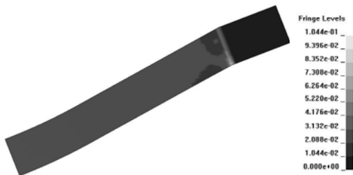
Fig.11 Plastic strain distribution by flexible die with urethane pad
