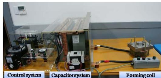
Fig. 9 Electromagnetic forming apparatus
