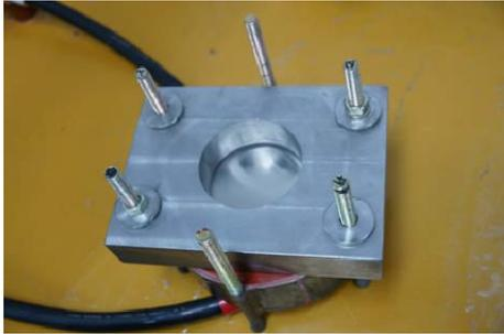
Fig.11 Assembly of forming coil and die
