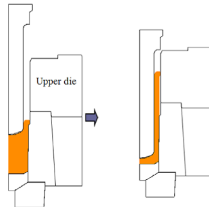
Fig. 4 Result of F.E analysis for final forging
