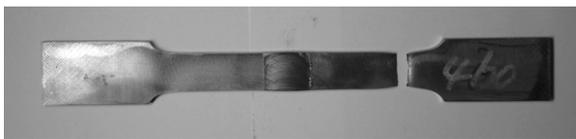
Fig. 9 Fractured tensile specimen of the friction stir welded 2205 duplex stainless steel
