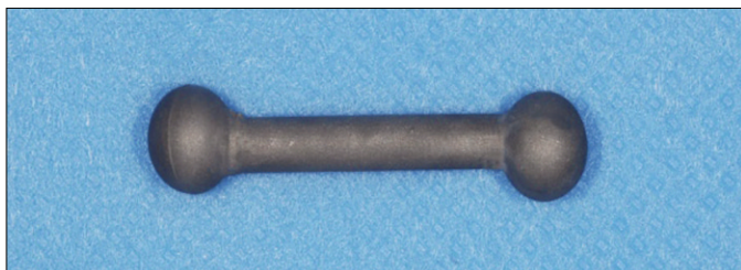
Fig. 1. The specimen made with Ni-Cr alloy.
