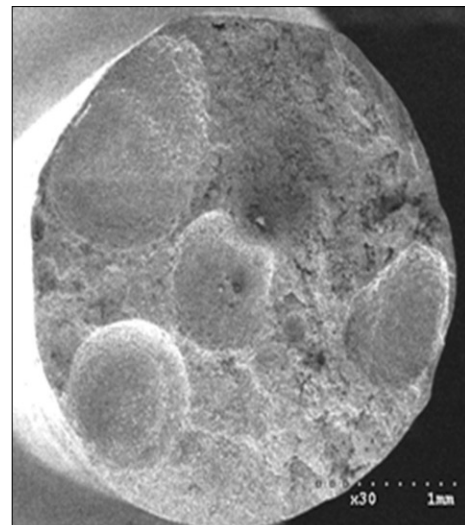
Fig. 4. SEM image of fracture surface of specimen ( \times 30 ).
