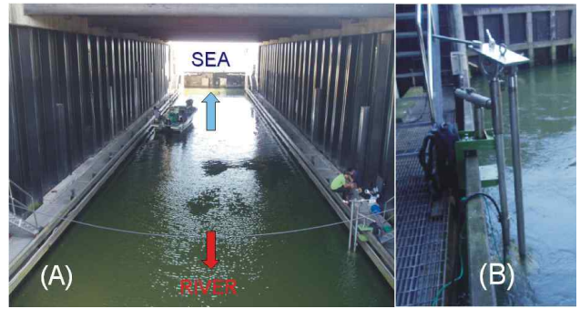
Fig. 2. Ship gateway through the Nakdong river (A) and monitoring rotator of an acoustic camera (B).
