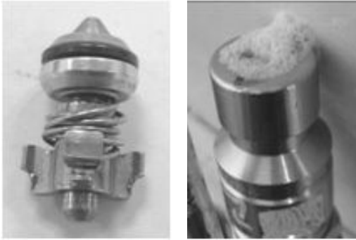
Fig. 10. Photographs of a leaking receptacle (left) and a damaged spring(right).
