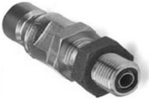
Fig. 1. Photograph of a typical receptacle used in CNG vehicles.
