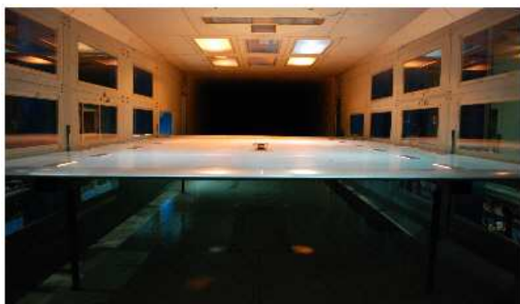
Fig. 20 The ground plate for wind tunnel test
