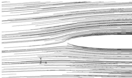
Fig. 12 Streamline of the leading edge at flap angle 0°
