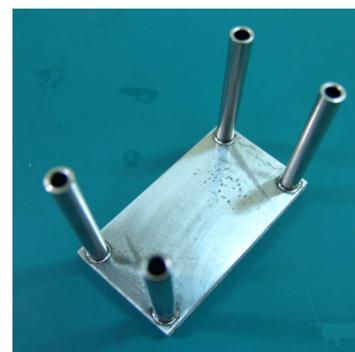
Fig. 3 Photograph of a micro-channels heat exchanger
