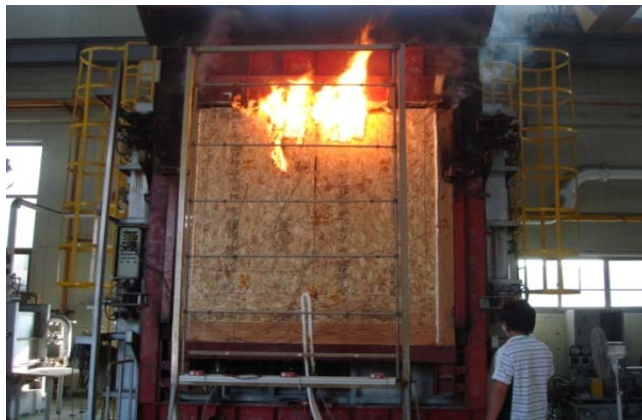
Fig. 7. Flame occurrence in light timber framed wall(38mm×140mm studs) reinforced by heavy timber frame after 80 minutes of fire exposure.
