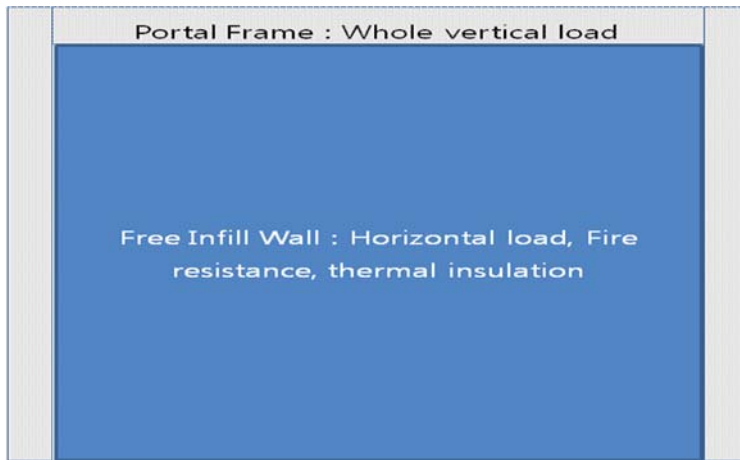
Fig. 1. Design concept of hybrid timber framed wall system.
