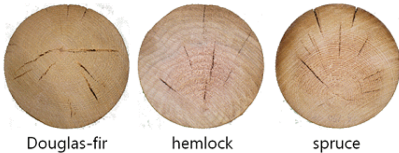
Fig. 5. Photos of three species roundwoods of 148mmΦ heat-treated at 170°C.
