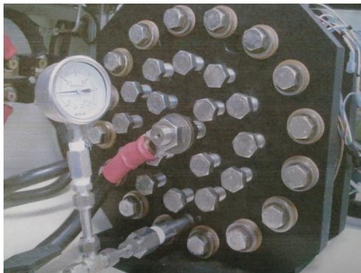
Fig. 2. Electrolytic cell is configured to produce bipolar plate.
