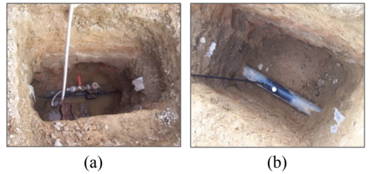
Fig. 3 Experimental set-up for leak locating tests of the plastic pipe (a) Leak valve, (b) Installed accelerometer
