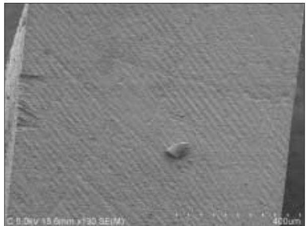
Figure 4. SEM micrograph of dentin side showing a representative adhesive failure of Maxcem along dentin surface ( \times 130 ).
