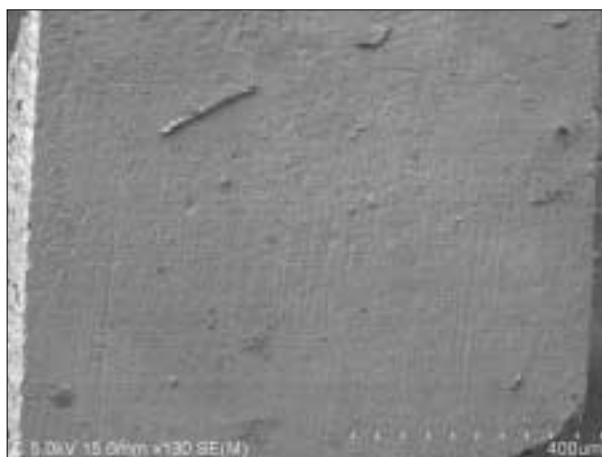
Figure 6. SEM micrograph of dentin side showing a representative adhesive failure of BisCem along dentin surface ( \times 130 ).
