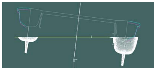
Fig. 7 Hull section with heel 7 deg.
