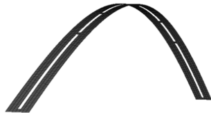
Fig. 4 Finite element model of a blade
