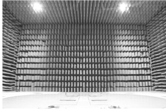
Fig. 3 Absorber-lined chamber for test
