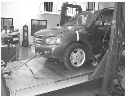
Photo. 3 Measurement of C.G.H in VCGM system
