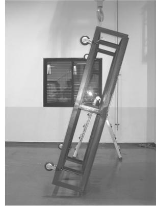
Photo. 2 C.G.H measurement for calibration fixture by gravity method
