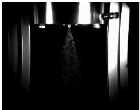
Fig. 10. Kerosene injector cold flow test
