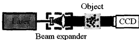
Fig. 1 Principle of in-line digital holography
