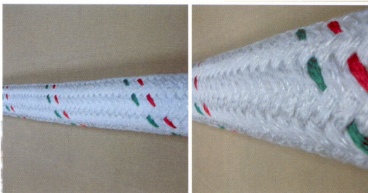
Fig. 3 Fiber rope with partial fluorescent painting
