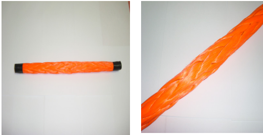
Fig. 2 Fiber rope with painting by fluorescence
