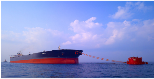
Fig. 6 SBM used floating hawser
