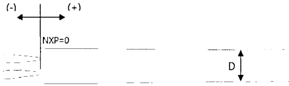
Fig. 3 Definition of primary nozzle exit position(NXP)
