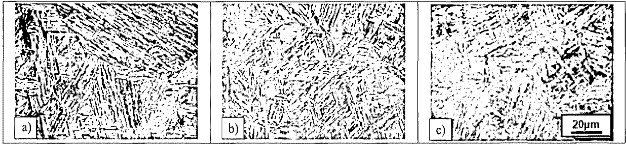
Photo 3 OM microstructures showing the effect of forging starting temperature in 9Cr-1Mo steel Forging starting temperature : a) 1150°C b) 1200°C c) 1250°C
