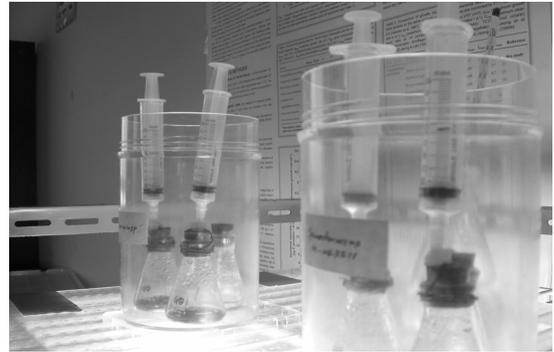
Fig. 3 Experimental setting for H<sub>2</sub> photo-production.
