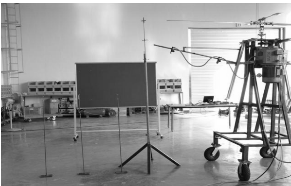
Fig. 2 Equipment for measuring application loss of spraying droplets by vortex flow and dawnwash.
