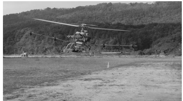
Fig. 6 Spraying test in the field using unmanned helicopter.
