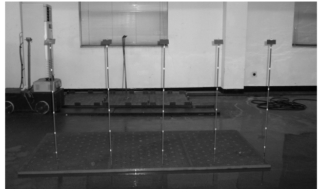
Fig. 3 Equipment for measuring vertical flow of spray droplets.
