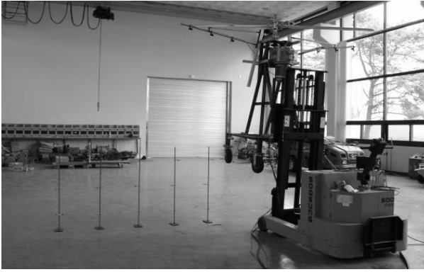
Fig. 1 Application characteristics test equipment by dawnwash of main rotor.
