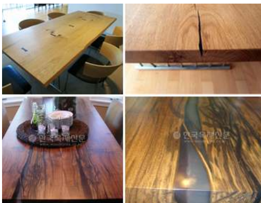
Fig. 2. Wooden Table(above) manufactured by reproducing Shake • Gnarl through Ebony Wood Powder Inlay Technique(Heukdan Mokbun Sangam Technique and Wooden Table(below) manufactured by reproducing Shake with Acrylic Resin. 8)
