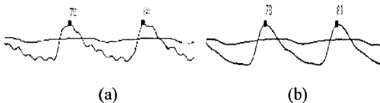
Fig. 2 Artifact removed PPG signal by shift mean distance treatment ((a) PPG signal including artifact, (b) PPG signal removed artifact)
