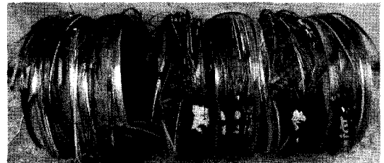
Fig. 14 Failure mode of Φ157.0(mm) hoop ring.
